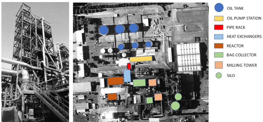
Fig. 5 Milling tower (left) and plan view of the Black Carbon Plant (Right)
