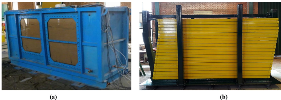
Fig. 1 Containers constructed and used in this study: a the rigid box, and b the laminar shear box
