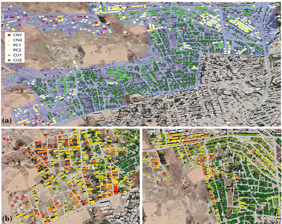
Fig. 12 Post-earthquake damage assessment for one typical block of buildings
