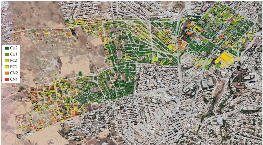
Fig. 11 A detail of Mila city’s building usability rating
