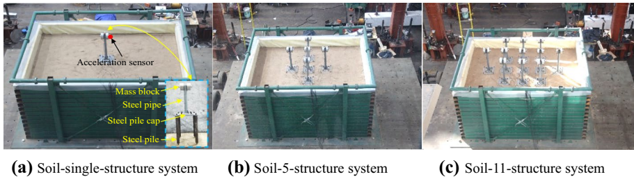
Fig. 2 Field photos of shaking table tests (Wang et al 2022a)
