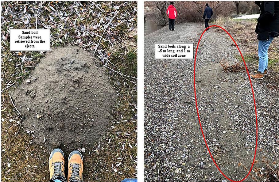
Fig. 8 Sand boils observed at Site 8 ( 38^{\circ}27'49.7''\text{N} 39^{\circ}24'01.1''\text{E} /31.01.2020/14:38 & 38^{\circ}27'49.8''\text{N} 39^{\circ}24'03.0''\text{E} /31.01.2020/14:14)
