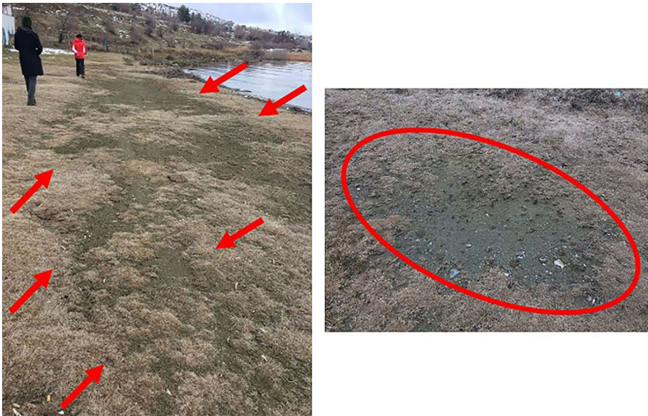
Fig. 9 Sand boils observed at Site 12 ( 38^{\circ}29'58.5''\text{N} 39^{\circ}30'24.6''\text{E} /31.01.2020/15:29 & 38^{\circ}29'57.7''\text{N} 39^{\circ}30'24.0''\text{E} /31.01.2020/15:30)
