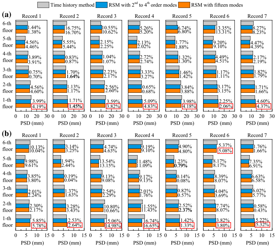
Fig. 11 Peak values of story drifts (PSD) of 6-story structure on a Site 1 and b Site 2 using Model 3 with accurate LPMs under artificial ground motions
