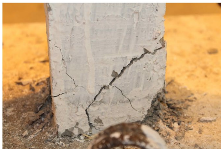
Story Drift = 3.73%: Concrete cover spalling and core concrete tension splitting.
