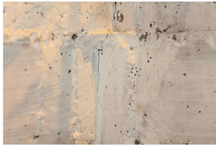
Story Drift = 1.10%: Flexure yielding of beam under connection closing.
