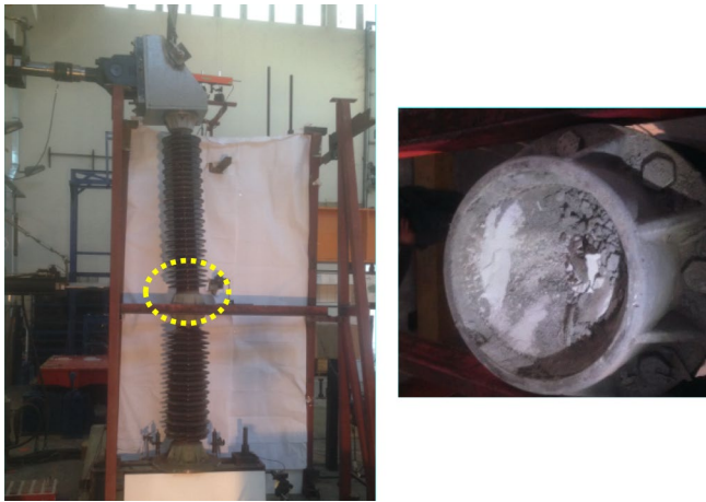
Fig. 12 The failure mechanism
