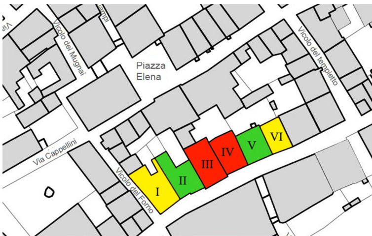
Fig. 14 Aggregate case study: MSU location and usability rating
