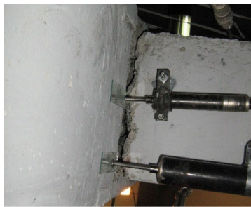
Fig. 11 Opening of the crack at the intersection of the beam and column
