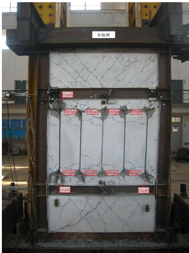
Fig. 9 Failure photo of specimen S-SLW
