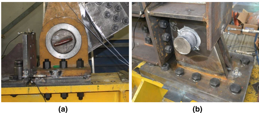
Fig. 3 Base connections of two specimen types. a PC specimen, b MRF specimen
