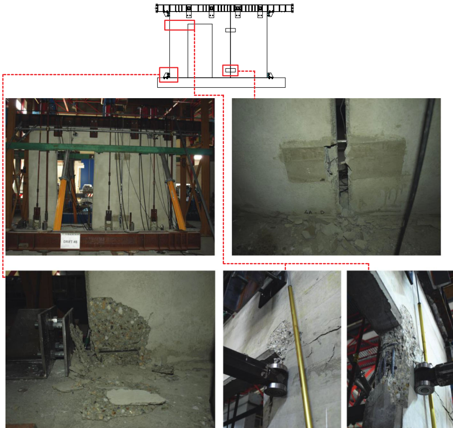
Fig. 17 Damage mechanism of specimen 07: deformed shape at the end of the test—detaching and pounding between wall segments ( top left ); failure of wall-to-wall connection systems ( top right ); concrete spalling and crushing at the base of the wall ( bottom left ); concrete crushing and buckling of longitudinal rebars at the corner of the door ( bottom right )
