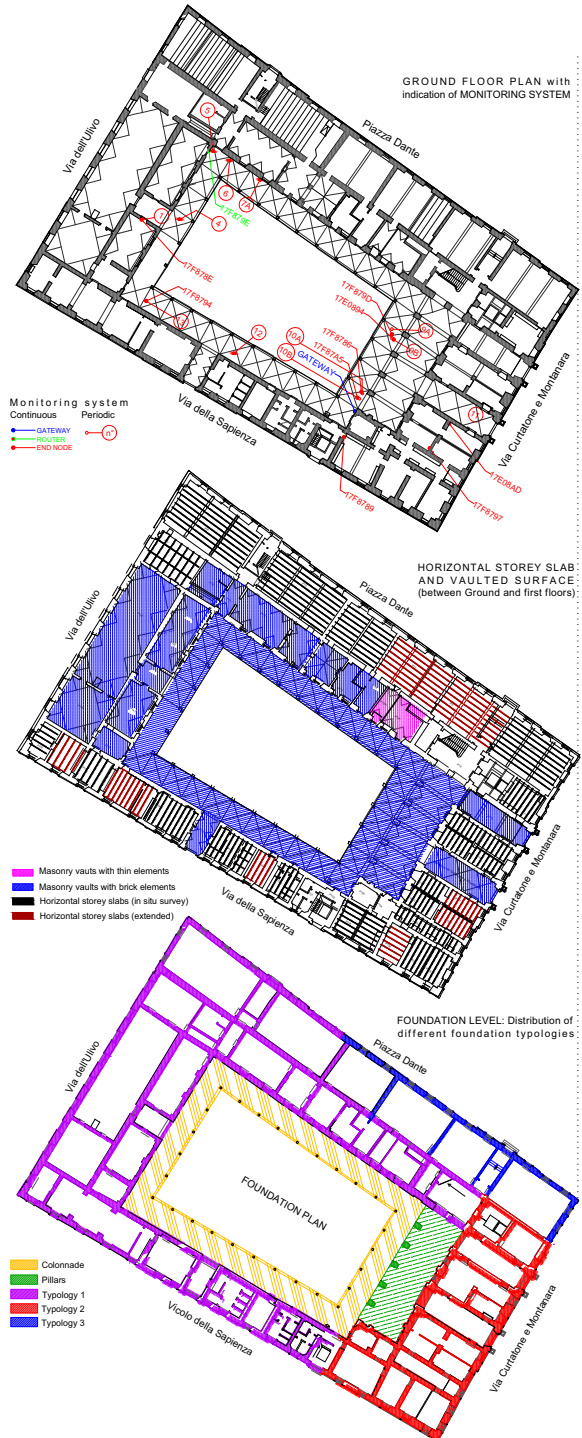
Fig. 10 Distribution of the floor slabs and types on the building's ground floor, Foundation plan, different typologies evidenced and ground floor plan with indication of monitoring points (continuous and periodic systems)
