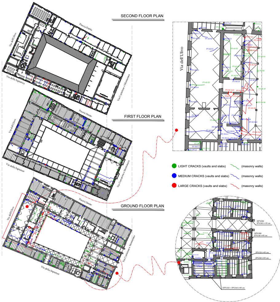
Fig. 11 Description of the cracking scenario at the different floors of the building
