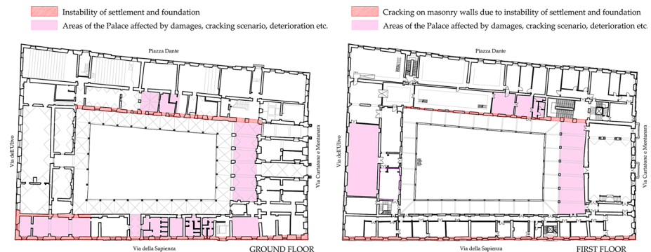
Fig. 7 Areas affected by problems and structural deterioration between the eighteenth and nineteenth centuries
