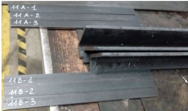
Fig. 13 Samples extracted from angular profiles of the braces for tensile tests
