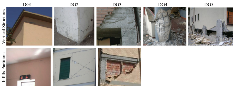
Fig. 8 EMS-98 DGs to Vertical Structures and Infills–Partitions
