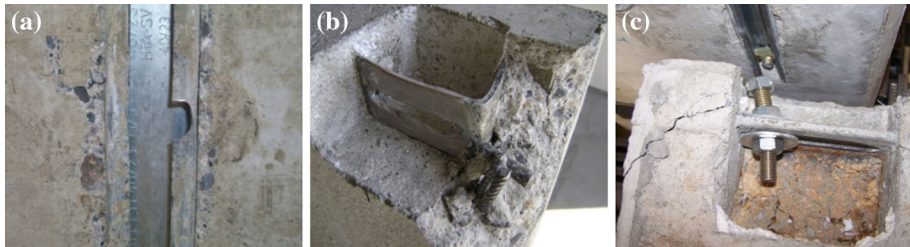
Fig. 6 Top connection failure mechanisms: a PCS A, b PCS B and c PCS D
