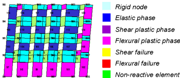
Fig. 9 Damage pattern on the back façade of the “Pombalino” building for the uniform load
