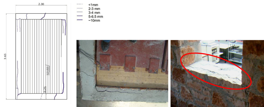
Fig. 18 PBM-As built specimen (BS). Observed damages at the roof level and at the level of openings after Test 8BS (Kalamata earthquake: 0.29 g(X)/0.24 g(Y), Table 4)
