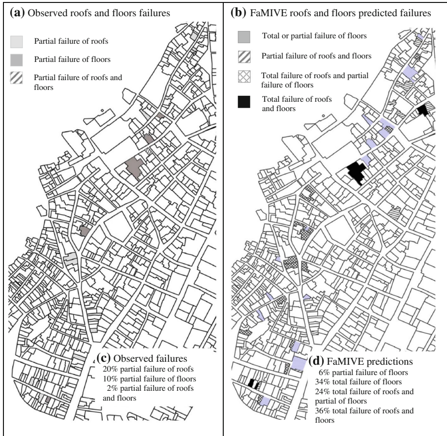
Fig. 18 Observed and predicted roofs and floors failures
