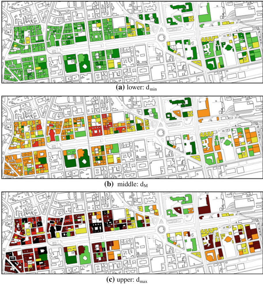
Fig. 9 Damage level in Habib Bourguiba computed according to the Eq. 2 and corresponding to EMS98 intensity 7
