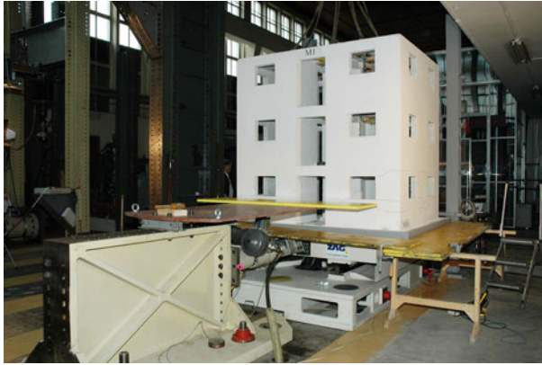
Fig. 14 Simple shaking table at ZAG with model M1 ready for testing
