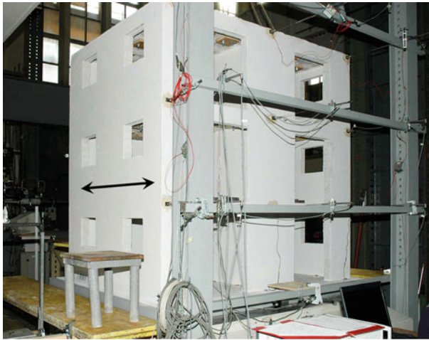
Fig. 18 Instrumentation and position of model M1 on the shaking table
