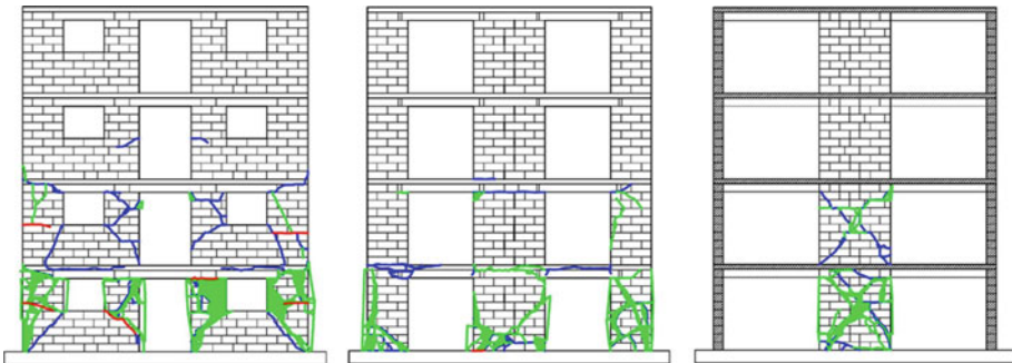
Fig. 21 Propagation of damage to the in-plane loaded walls of model M3 at damage limit ( red ), maximum resistance ( green ) and ultimate state ( blue ). Storey failure mechanism is clearly visible
