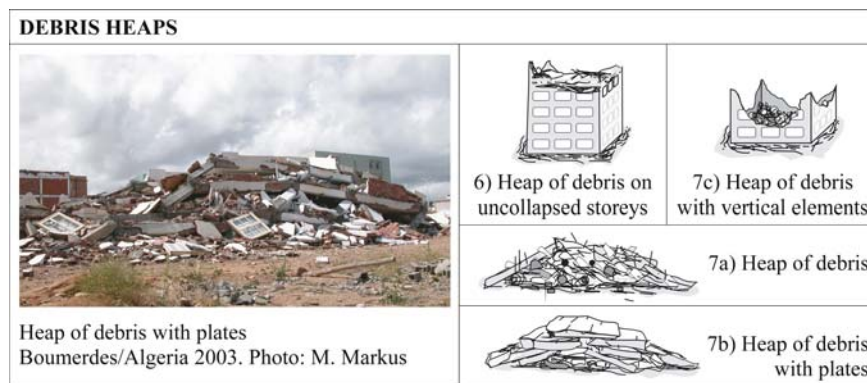
Figure 4. Damage type group – Debris heaps.
