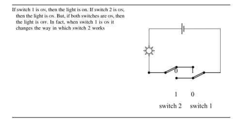
Now, two men are sent for turning the light on. The task of the first one is to switch  $S_1$  on, while the task of the second one is to switch  $S_2$  on just in case the first man does not achieve his task. Let's assume that the first man has success. The causal model looks as follows:
