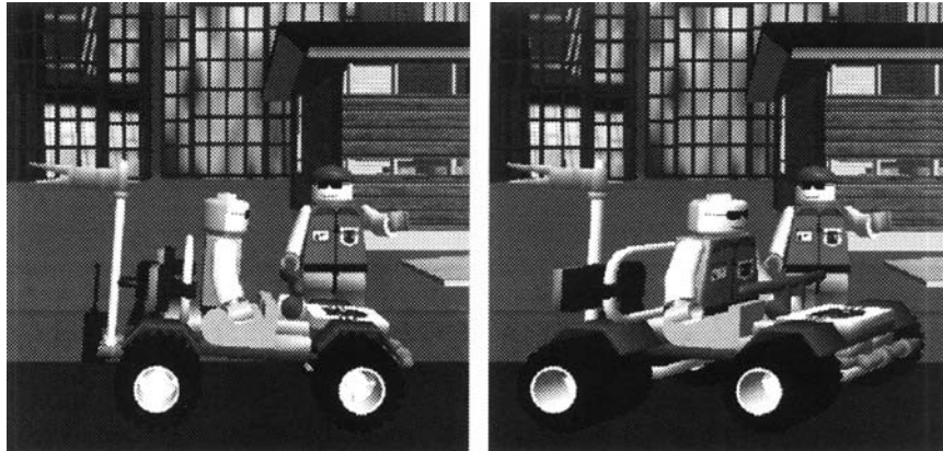
Figure 11. Single vs. multiple projections. The left image is a classic linear perspective view. The right image uses multiple projections, and each object is assigned a different drawing(spatial) system. The background house is depicted using linear perspective to convey a sensation of depth, while the car and foreground character are represented using oblique projection to enhance the visibility of the character's face. Image courtesy of Maneesh Agrawala.
