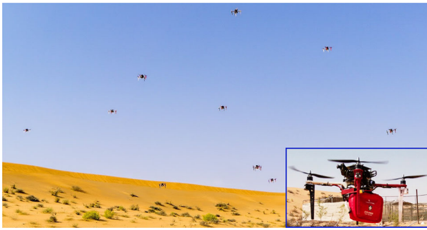
Fig. 1 UAV swarm exploring a desert environment in a decentralized search and rescue task without wireless communication among the robots
