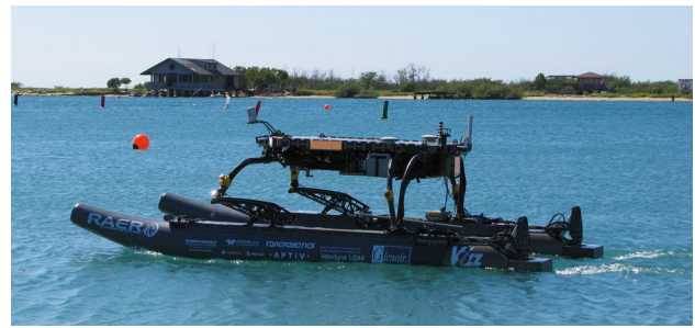
Fig. 7 The Minion Research Platform is a 16-foot long USV that is equipped with a high fidelity GPS/INS and four multi-beam Lidar sensors
