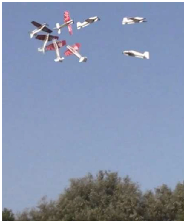
Fig. 14 Fixed-wing aggressive turnaround image sequence: the plane starts at the bottom right in level flight, pitches until inverted flight, and then rolls into level flight with the opposite heading
