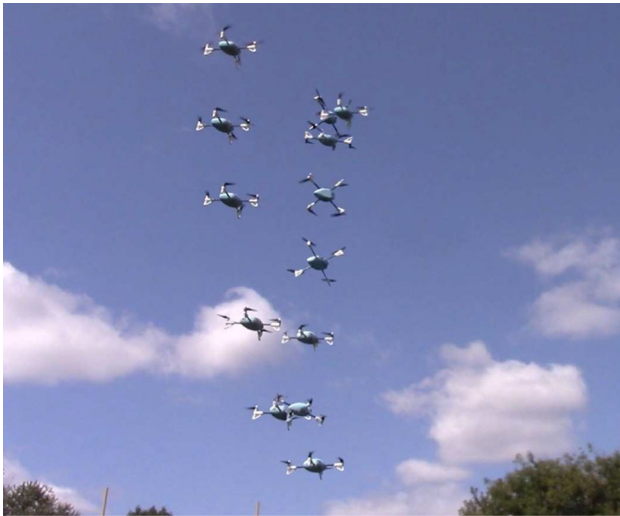
Fig. 11 Quadrotor rolling flip case 1 image sequence: the flip begins on the right side of the image, performs the flip while losing altitude, and then returns to the start of the maneuver
