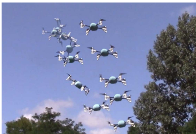
Fig. 12 Quadrotor Rolling flip case 2 image sequence: the flip begins on the left side of the image, performs the flip quickly, loses altitude, and then returns to the start of the maneuver
