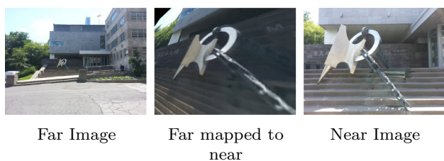
Fig. 1 A homographic mapping between two images computed using Object Landmarks , as described in Sect. 3.2. Despite a 6\times difference in visual scale, the highly-distinctive foreground object allows our system to determine an accurate homography between the images. See also Fig. 8
