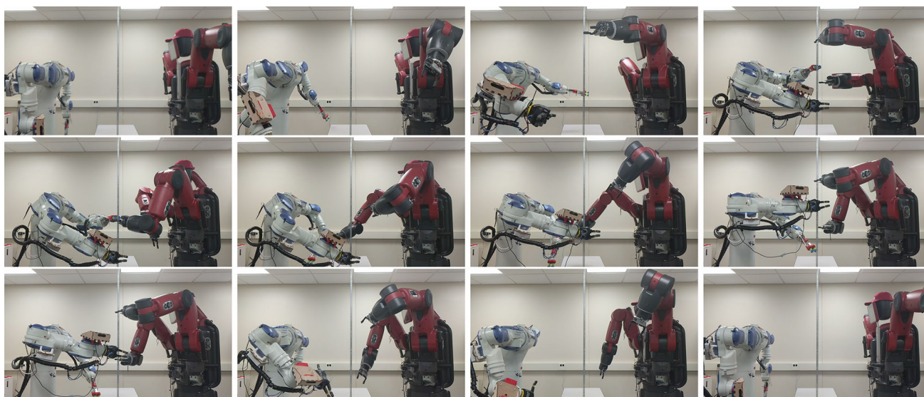
Fig. 19 Real world experiments were performed in a 28 dimensional space with 2 dual-armed manipulators planning their motion from a start state to an approach state close to a pole positioned in the center of a tightly coupled shared workspace. The arms then swap positions
