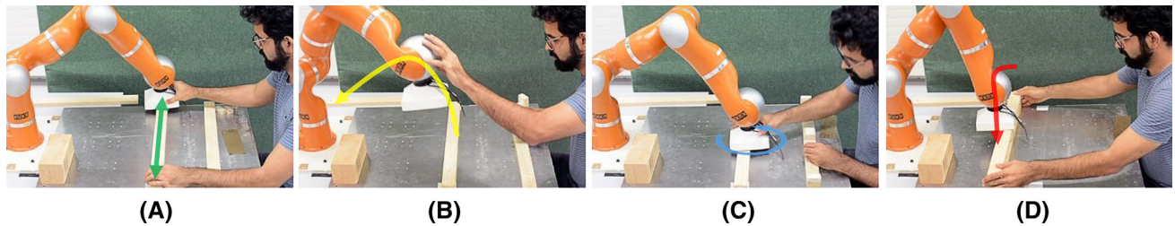
Fig. 8 An example of task-adaptation in compliant human–robot interaction. The user and the robot perform a series of manipulation tasks jointly. The robot recognizes the intention of human and adapts its
