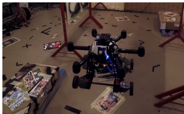
Fig. 10 AscTec NEO hexacopter equipped with a dual arm manipulator along with a specially designed lightweight UGV
