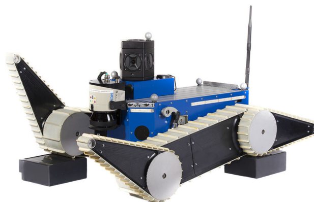
Fig. 13 TRADR UGV equipped with multiple encoders, an IMU and a rotating laser-scanner
