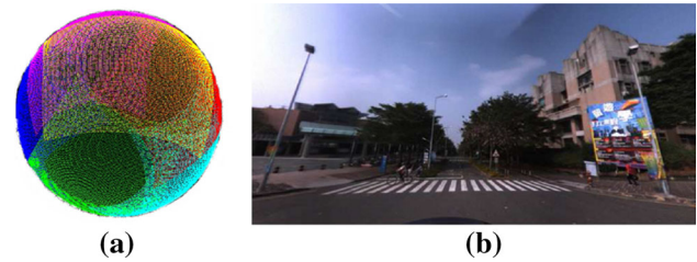
Fig. 10 3D spherical surface mapping used to synthesize a perspective image from six outward camera views. a The different colors represent the mesh points of individual cameras. b An image cropping result from the Ladybug2 six-camera imaging
