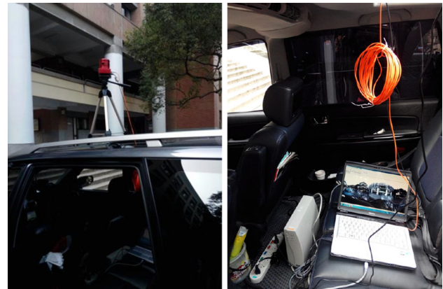
Fig. 13 The camera is mounted on top of a vehicle for image acquisition
