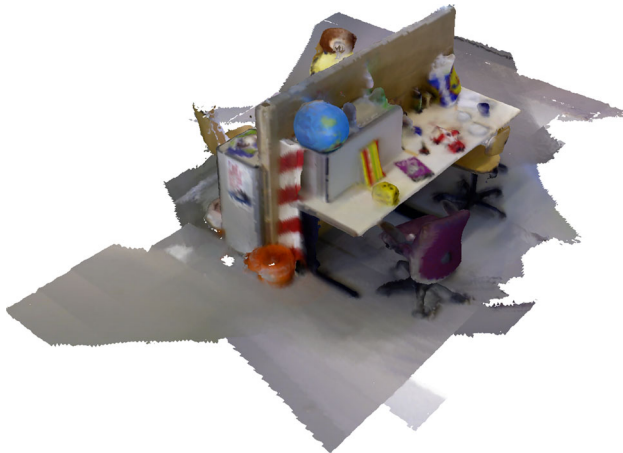
Fig. 20 Reconstruction using the Freiburg desk public dataset Sturm et al. (2012) , based on the motion-capture ground-truth trajectory. The maximum depth used is 2 m. Performed on a desktop machine
