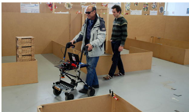
Fig. 22 Blind user and the experimenter in the test environment for the pilot study. The participant is currently walking on the main floor. Two small floors and the adjacent rooms can be seen in the background
