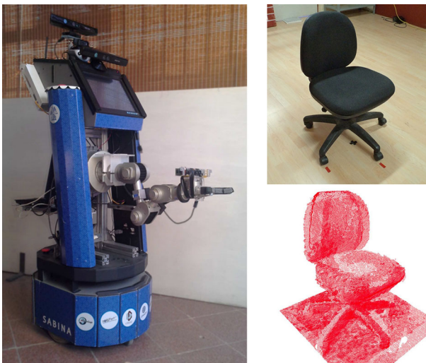
Fig. 1 The proposed method is able to plan each robot view/state in order to reconstruct a real object. In our experiments we use a mobile manipulator of 8 degrees of freedom to reconstruct several objects. A Kinect sensor was mounted on the robot's end effector
