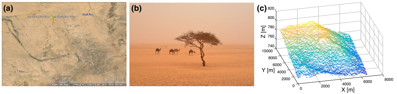
Fig. 5 Sahara desert (Chad, Africa). SRTM DEM (90-m resolution). a Overhead view (Google Earth). b Detail of this environment. c DEM, raw samples (color represents elevation)
