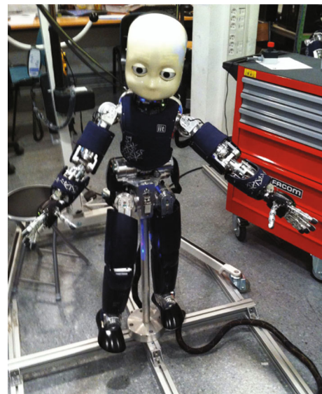
Fig. 9 The iCub robot being controlled by the proposed approach to perform a head position task, a left hand position task, a posture task, and a joint limit avoidance task
