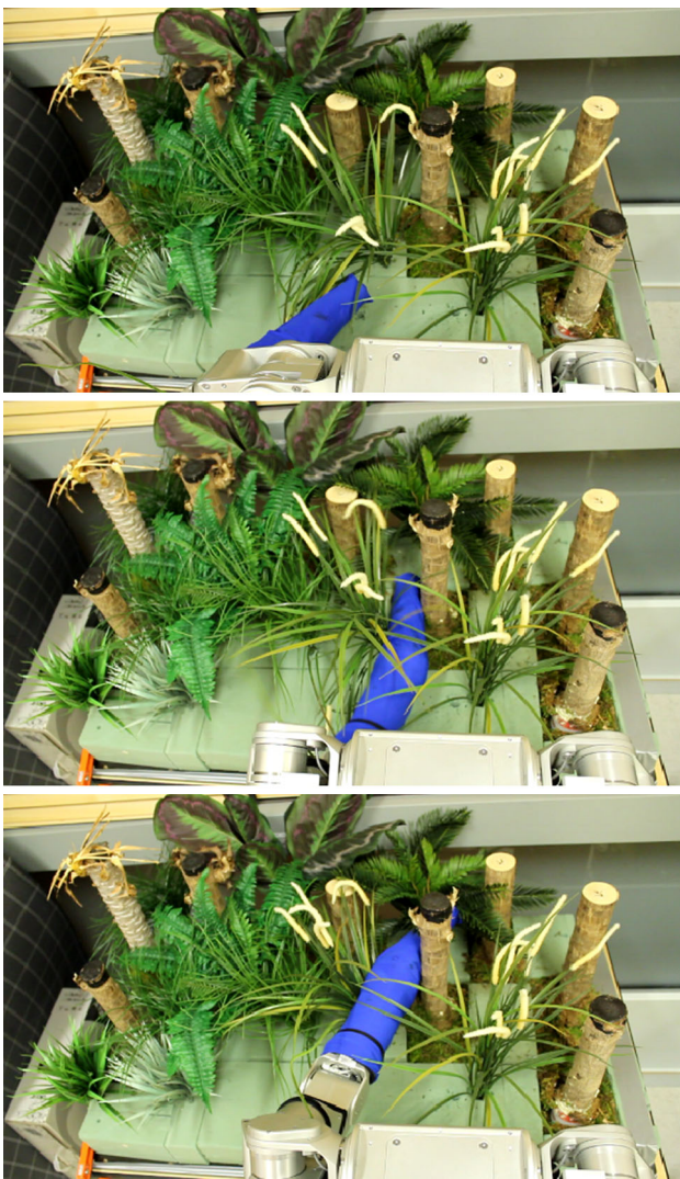
Fig. 13 Sequence of images from one trial out of 105 trials where DARCI reached into simulated foliage while controlling estimated contact forces using dynamic MPC
