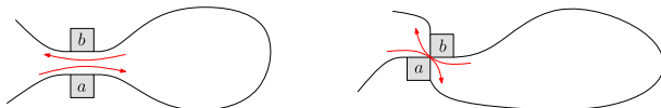
Fig. 15 Two possible bottleneck types created by a pair of co-vertical modules (left) or a pair of modules sharing a vertex (right). Arrows indicate the directions in which modules may attempt to move through the bottleneck
