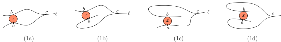
Fig. 17 The four possibilities in a bottleneck configuration if c is distinct from a and b . In all cases, module x applies a jumping rule, i.e., it changes attachments from a to b . The letter \ell indicates the topological position of the leader of the configuration
