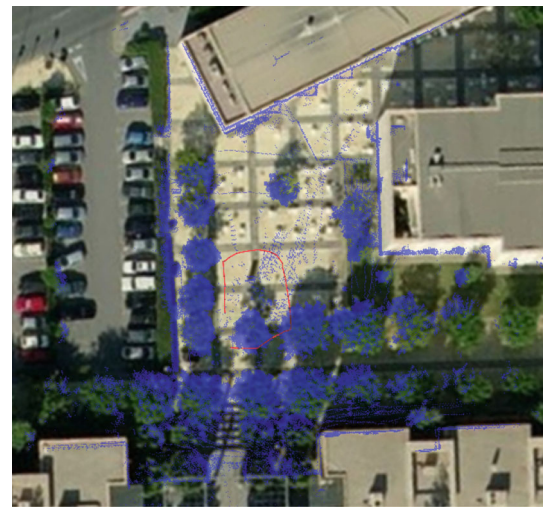
Fig. 9 Zenithal view of the resulting map of the Polytechnic College data set experiment using a 3D laser. Map points are superimposed to a real aerial picture. The red line represents the computed robot trajectory (Color figure online)
