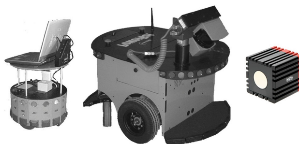
Fig. 2 Two robots used in this paper together with different 3D devices: from left to right, a stereo camera, a 3D sweeping laser and a SR4000 camera
