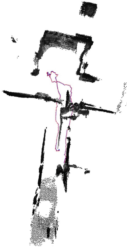
Fig. 8 Indoor map building experiment using a SR4000 camera: zenithal view of the resulting 3D reconstruction. The red line shows the path follow by the robot (Color figure online)
