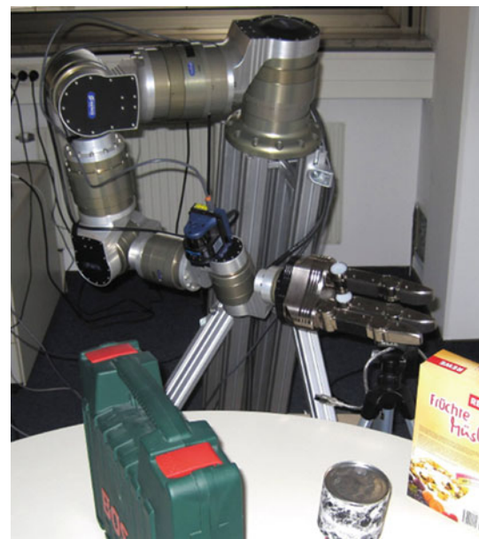
Fig. 9 The Schunk robot arm, the SDH hand and an arm-mounted Hokuyo URG-04LX laser
