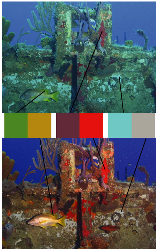
Fig. 1 Comparison of underwater imaging using white flash and adaptive illumination in a wreck setting. The color row in the middle shows color patches extracted from these images for visualization without the scene context. The images show a coral formation on a ship wreck in the Grand Cayman with existing white flash ( Top ) and adaptive illumination ( Bottom ). The pictures were taken at 15 m depth by Cathy Church. The scene was at a distance of 3 m
