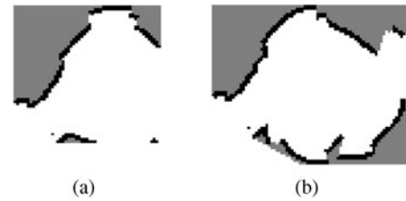
Fig. 11 Template grid maps: (a) inadequate template grid map for reliable grid-map matching and (b) template grid map expanded by accumulating more sensor data
