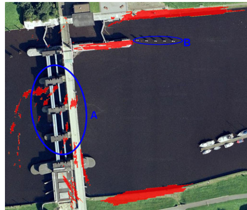
Fig. 29 Two environment parts that are not or only sparsely covered in the 3D map generated by plane-based registration
