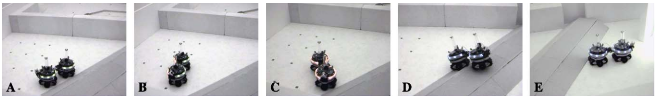
Fig. 12 Execution of the controller for the connected coordination strategy. (A): The s-bots have already aggregated and self-assembled as a response to having encountered the hill. The connected swarm-bot performs phototaxis and approaches the hill with an inappropriate (random) orientation. Having detected the hill, the swarm-bot performs antiphototaxis, with the result that it moves away from the hill. (B): The swarm-bot rotates until it has a more appropriate orientation (based on
