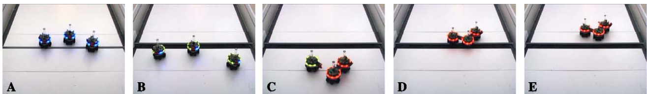
Fig. 15 The basic self-assembly response strategy in the hole crossing task. (A): s-bots cross a 3 cm hole individually. (B–E): s-bots respond to a 10 cm hole by self-assembling and crossing collectively.
