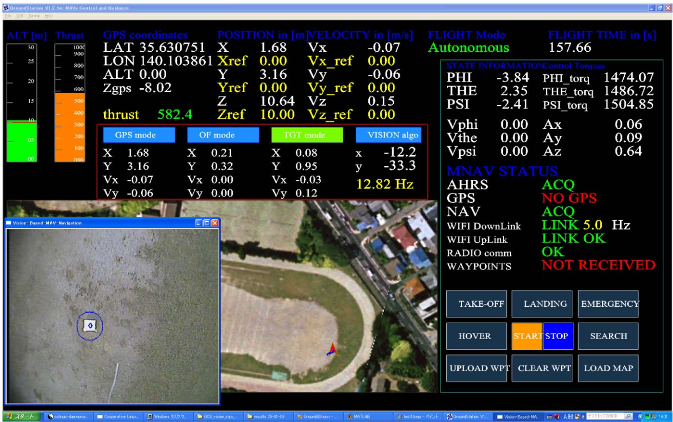
Fig. 6 The interactive interface of the ground control station during vision-based autonomous hovering
