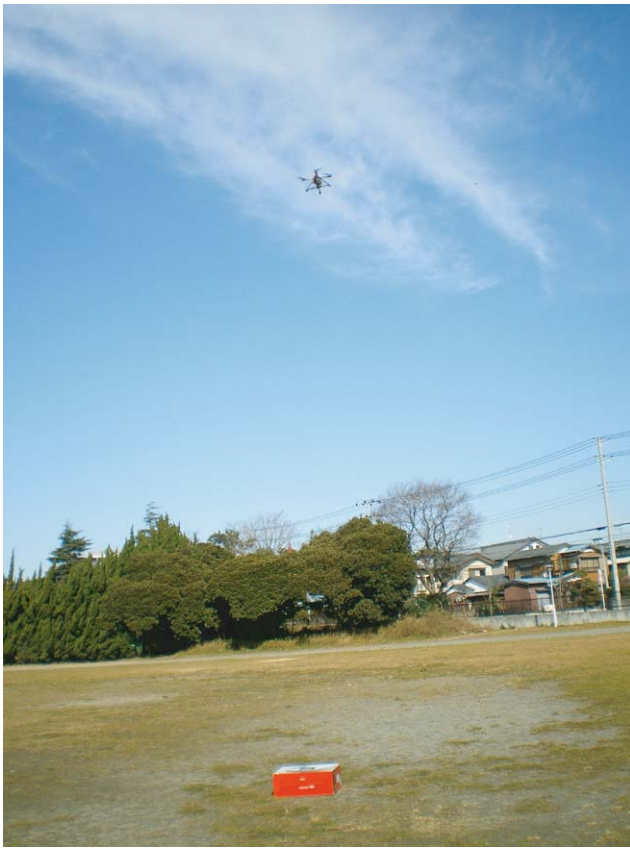
Fig. 11 Rotorcraft during vision-based autonomous hovering above a stationary target
