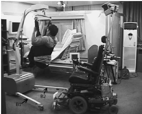
Fig. 14 Transfer of a user from the bed to the wheelchair
