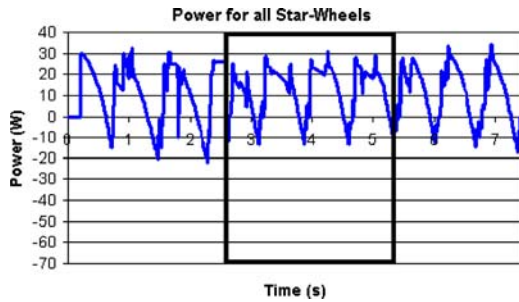
Figure 16. Consumption power for climbing six stairs.
