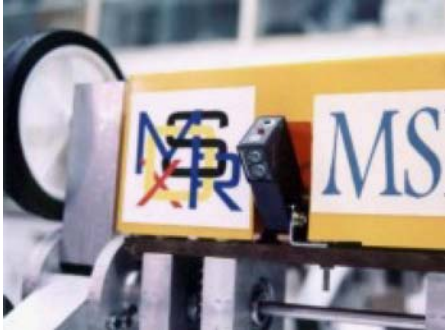
Figure 29. The MSRox's photoelectric sensor.
